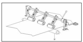
(Code: 3R1) Roller sensor unit for spun or woven fabrics, complete with lifting and mounting accessories.
